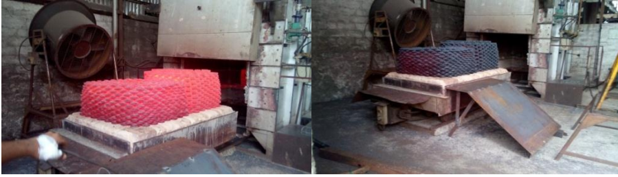
Figure 4.5 Ramp to unload hot components from bed
