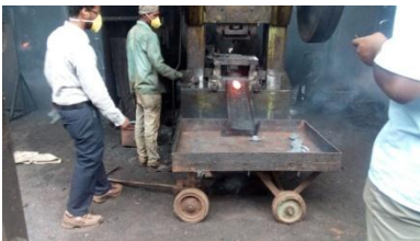
Figure 4.4 Direct collection of trimmed components in trolley
