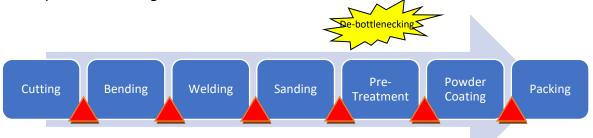
The overall conversion process includes a mix of manual and machine operations. The data taken clearly showed that the chemical pre treatment process prior to color coating was the bottleneck. However, observations made at the *gemba* gave a further insight – the pre treatment capacity itself is underutilized due to inconsistent supply of material from the preceding welding operation. Hence the roadmap made prioritized these projects
