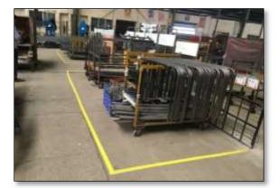
A kitting supermarket for fabricated components was established before welding – where all parts required for welding a sub assembly are brought. If any part is missing, the material feeder immediately follows up with the fabrication in charge to get it completed.
