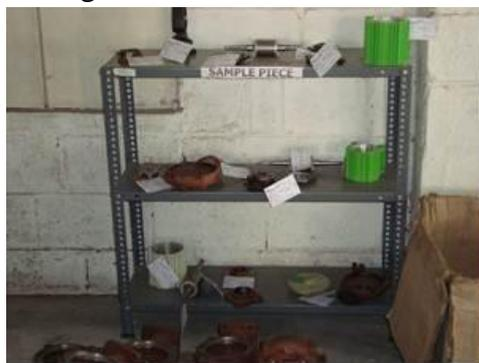
In Incoming Inspection, Master Samples of Incoming Components are (approved samples) displayed as ready reckoner.
