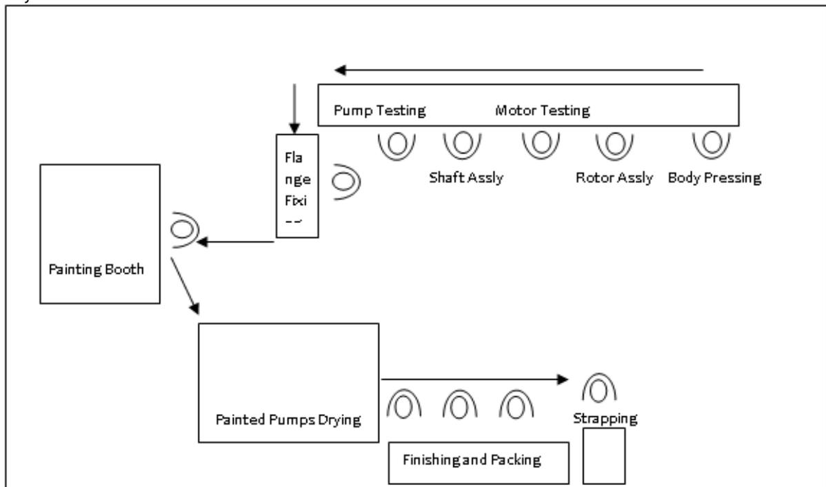
During the project, the demand for a new product (mini pump) increased considerably again doubling the requirement from the unit. There were significant differences between the process and sequence of new model and the regular ones resulting in the need for a new assembly and packing line. During the final stage of implementation, it was also decided to reduce the length of the existing line so that the strain for the
