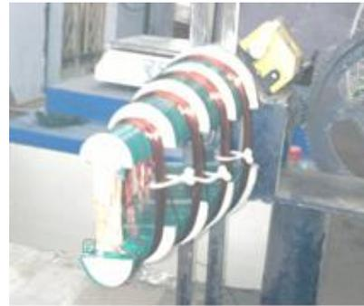
Introduced clamping of different rolls of coils at winding itself – making it easy for winding by eliminate tying with thread and eliminating mix
