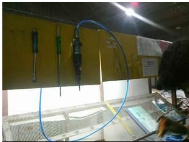
Workstations designed all the tools were arranged in the sequence of their use and to ease the pickup and use.
