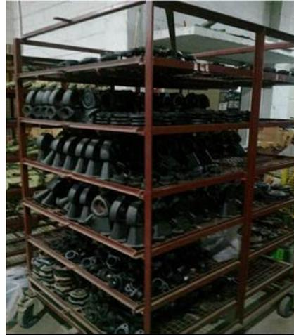
Multi-Layer storage provide with wheels (movable racks) saving space and eliminating the movement of operators'.
