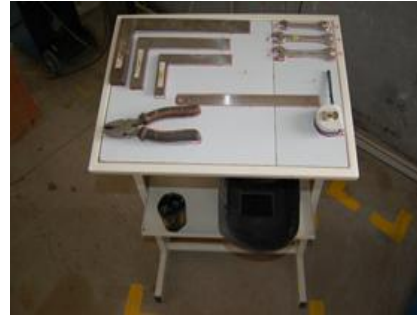
Tool board made and all tools placed in marked location making it search free and visible.
