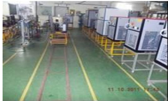
Flow line has been clearly marked and FIFO could be followed.
