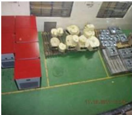
2) Dryer box arrives from sheet plant with the door screwed on, the assembler has to un-screw and remove the door for doing his work. The door is again rescrewed at the end of the line.
